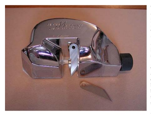
The Dexter is a hand held device which holds a blade positioned at a 45 degree angle so that your cut will be beveled. To cut simply measure and trace the opening as described above and use a straight edge ruler to guide the Dexter. Make sure that you over cut each side 1/4" approximately so that the opening will fall out after you are done cutting it. The over cut is necessary because the bevel makes the opening on the back of the mat slightly smaller that the opening on the front of the mat.
